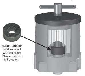
If the 500 Series filter assembly has this spacer installed, please remove it when using this redesigned replacement filter.
